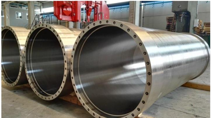
Vertically centricast items with OD between 300 and 1400mm, ID between 150 and 1350mm, lengths up to 1250mm. Vertical centricast items are normally shaped, but we can produce also simple cylindrical rings.
